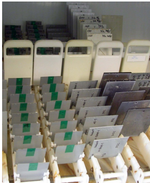
Fig. 6 Example of open and well drained fixtures for flat test panels (left) and minimum recommended stacking distance of panels (right)
